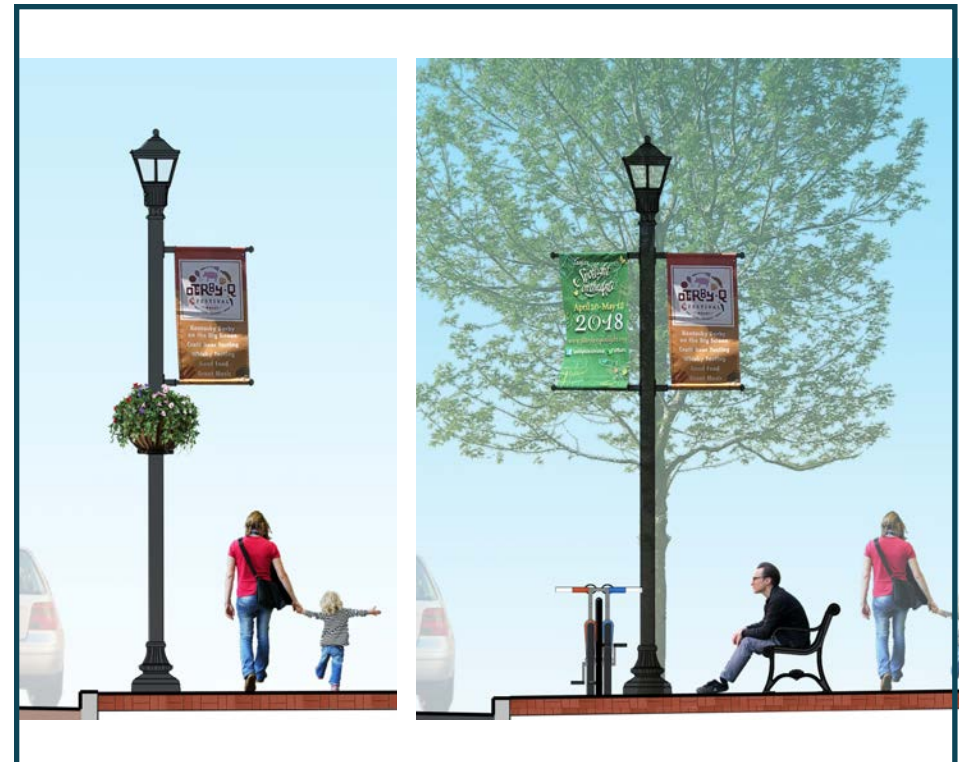
Pedestrian light with hayrack basket and single banner on left and double banners on right
