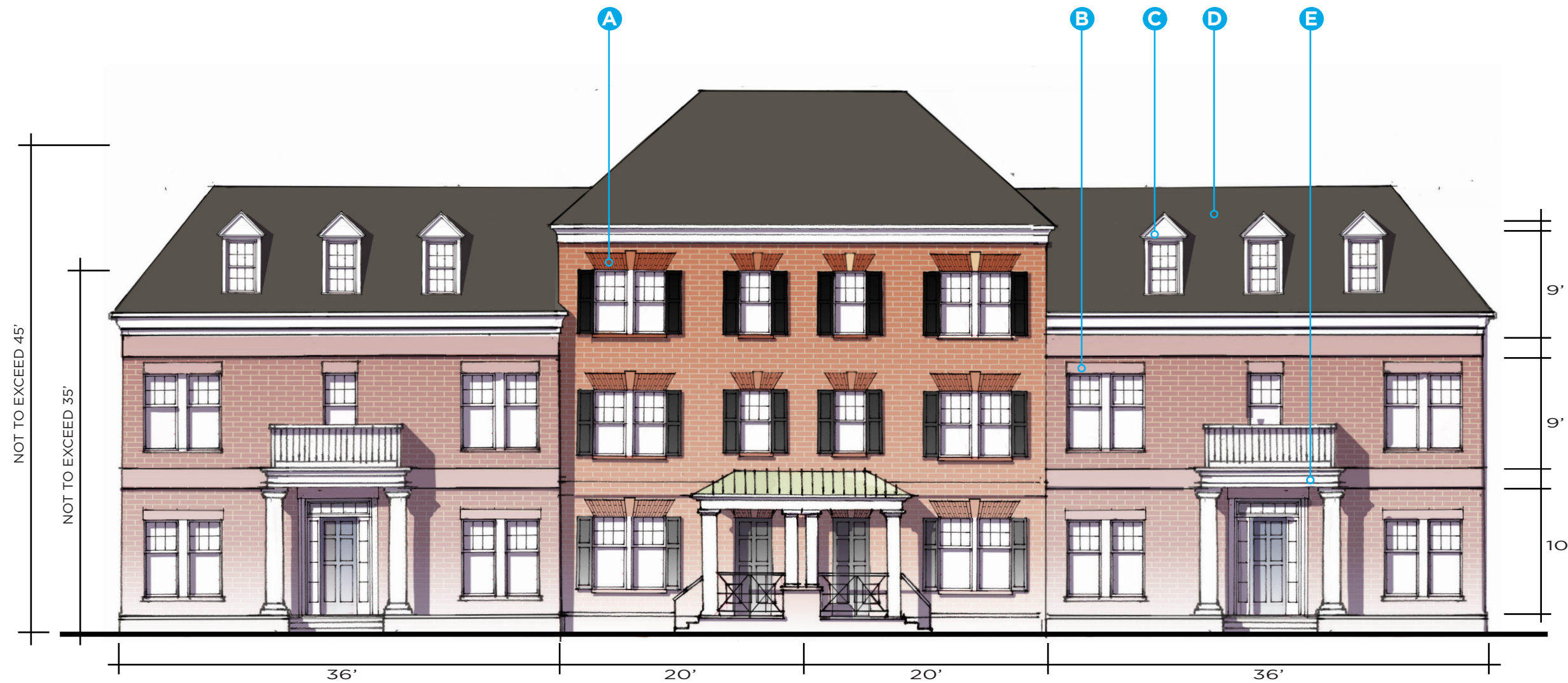
1 FRONT ELEVATION (STREET SIDE)
