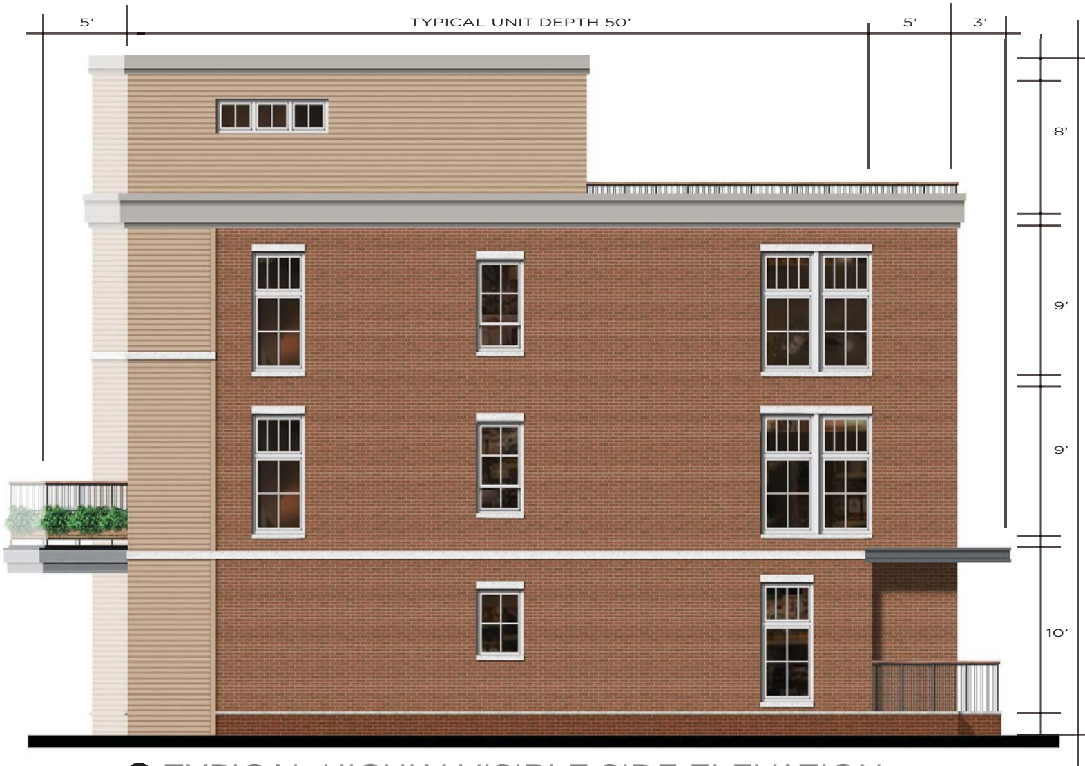
1 TYPICAL HIGHLY VISIBLE SIDE ELEVATION
