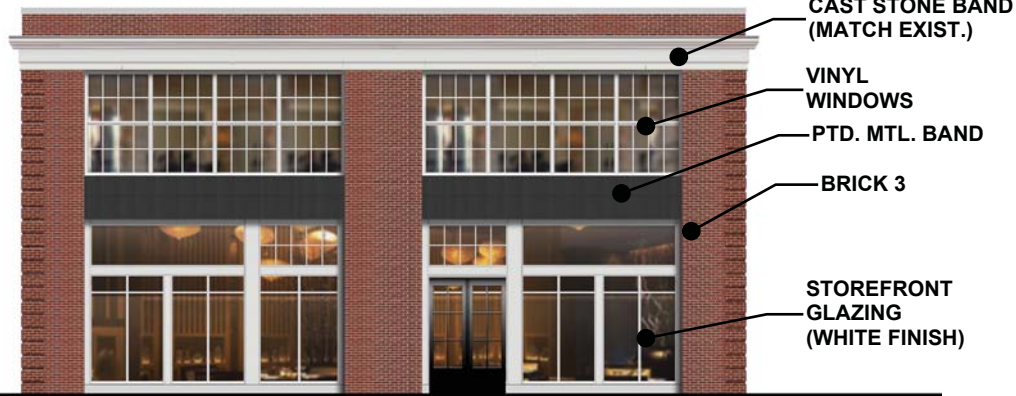
3 SIDE ELEVATION (EAST SIDE)
