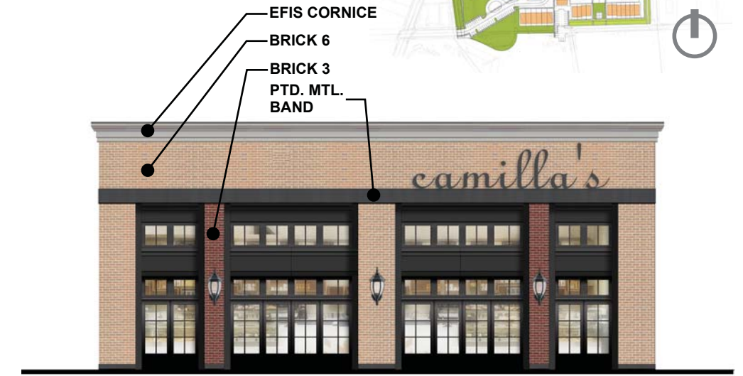
2 SIDE ELEVATION (NORTH SIDE)
