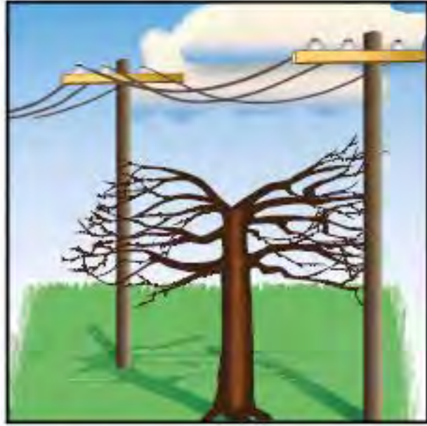
Natural lateral trimming for clearance under conductor area.
