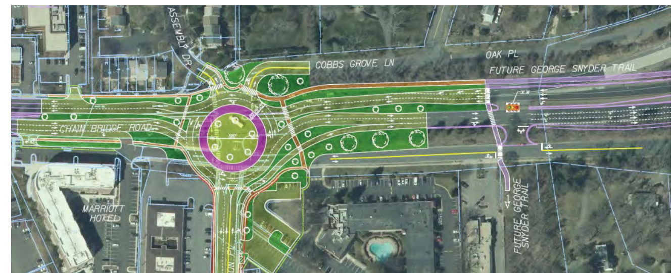
Figure 2. Proposed roundabout at the Chain Bridge Road/Eaton Place intersection (design developed by others)
