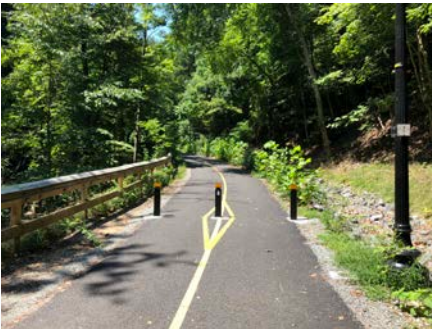
Typical bollard layout, with center removable bollard
