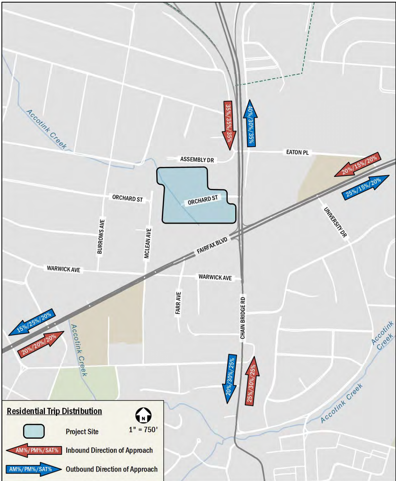
Figure 2: Direction of Approach for Residential Uses
