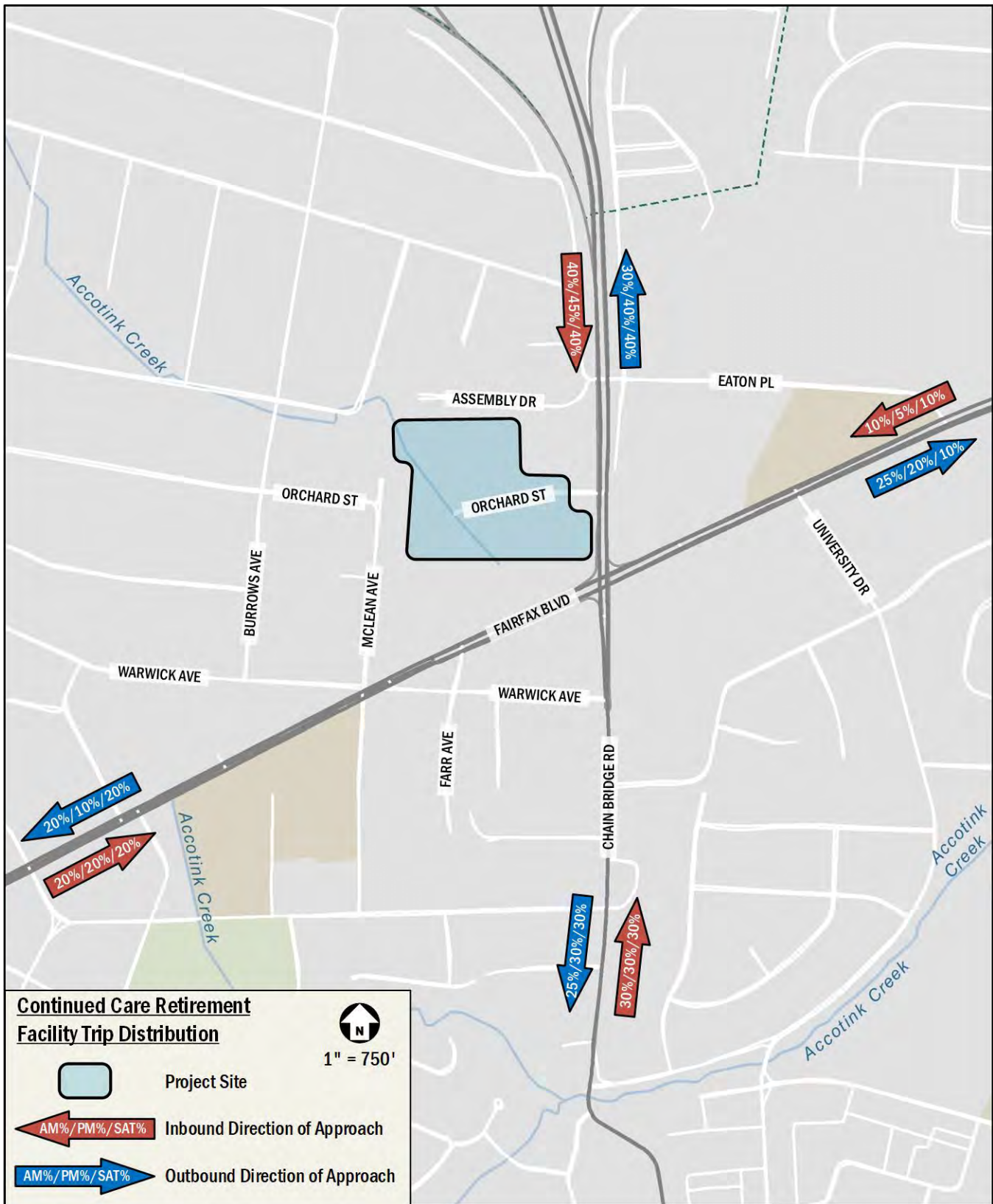
Figure 3: Direction of Approach for Continued Care Retirement Facility
