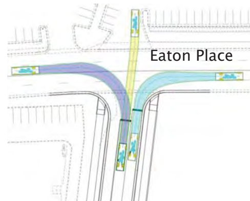
Intersection Turning Movements - Northfax East Roadway at Eaton Place
