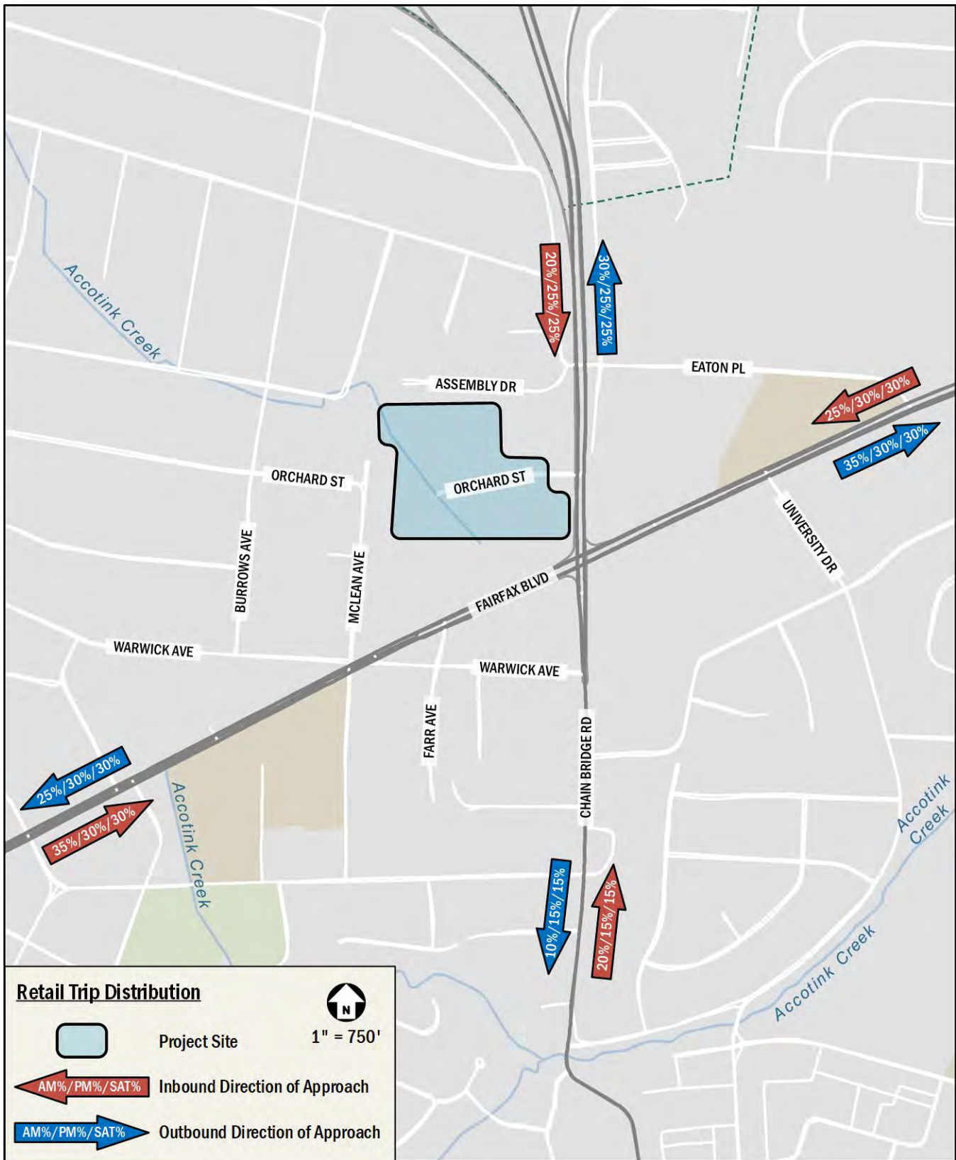
Figure 6: Direction of Approach for Commercial (Shopping Center and General Office)
