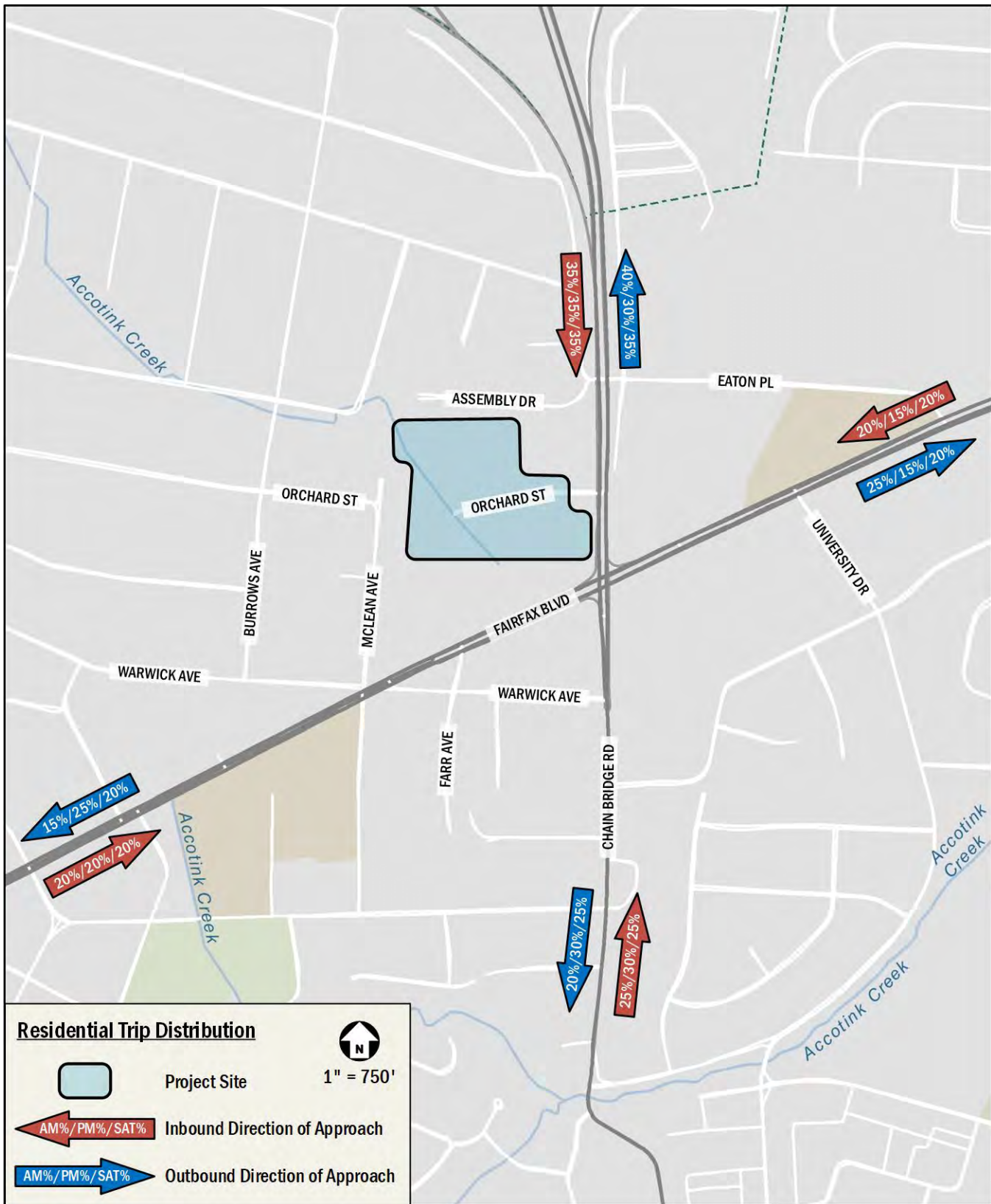
Figure 2: Direction of Approach for Residential Uses
