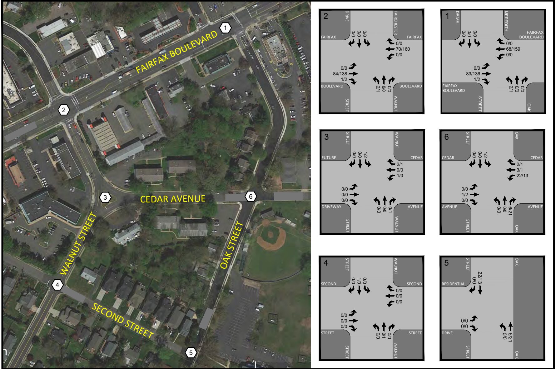
Figure 5-1 Pipeline Development Traffic Assignments Breezeway Property
