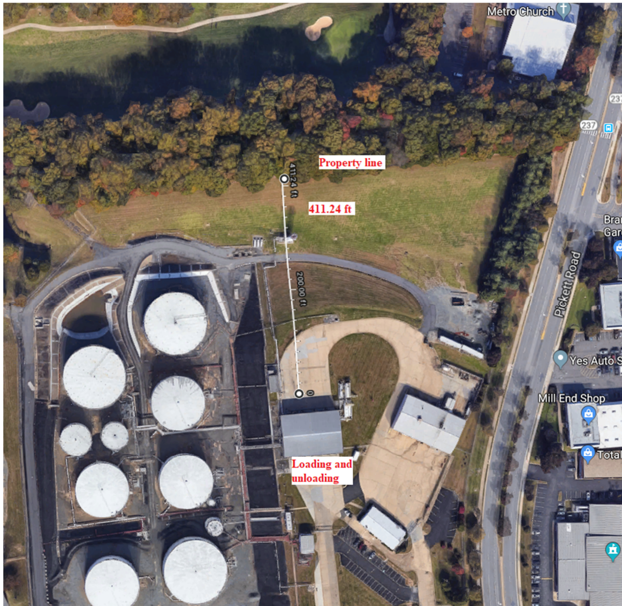
Figure 4 - Aerial view of the project site, showing actual distance between fuel loading / unloading area and the property line is approx. 411 ft
