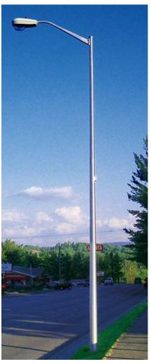
Smooth round tapered poles constructed of aluminum alloy for side mounted luminaires. Single arm or two arms at 180 degrees. Poles are directly embedded for use with underground supplied conductors only.
