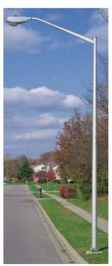
Smooth round tapered poles constructed of aluminum alloy for side mounted luminaires. Single arm or two arms at 180 degrees. Poles are base mounted for use with underground supplied conductors only. Anchor base poles require customer-installed and maintained concrete pole foundations and anchor-bolts.
