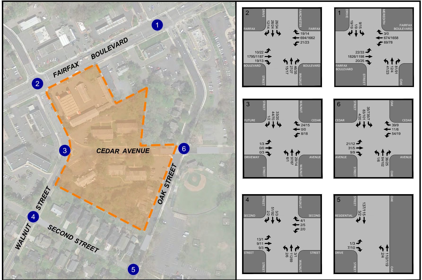
Figure 5-2 2024 Background Future Peak Hour Traffic Forecasts With Pipeline Developments
