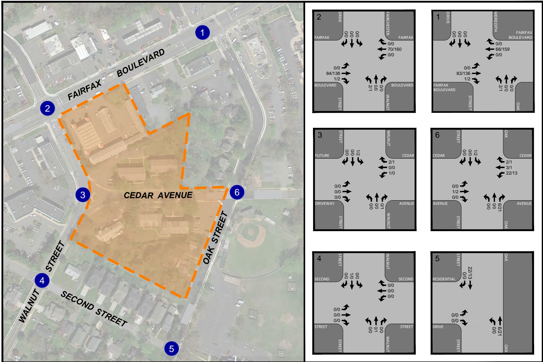
Figure 5-1 Pipeline Development Traffic Assignments Includes Novus Fairfax Gateway and Paul VI Redevelopment
