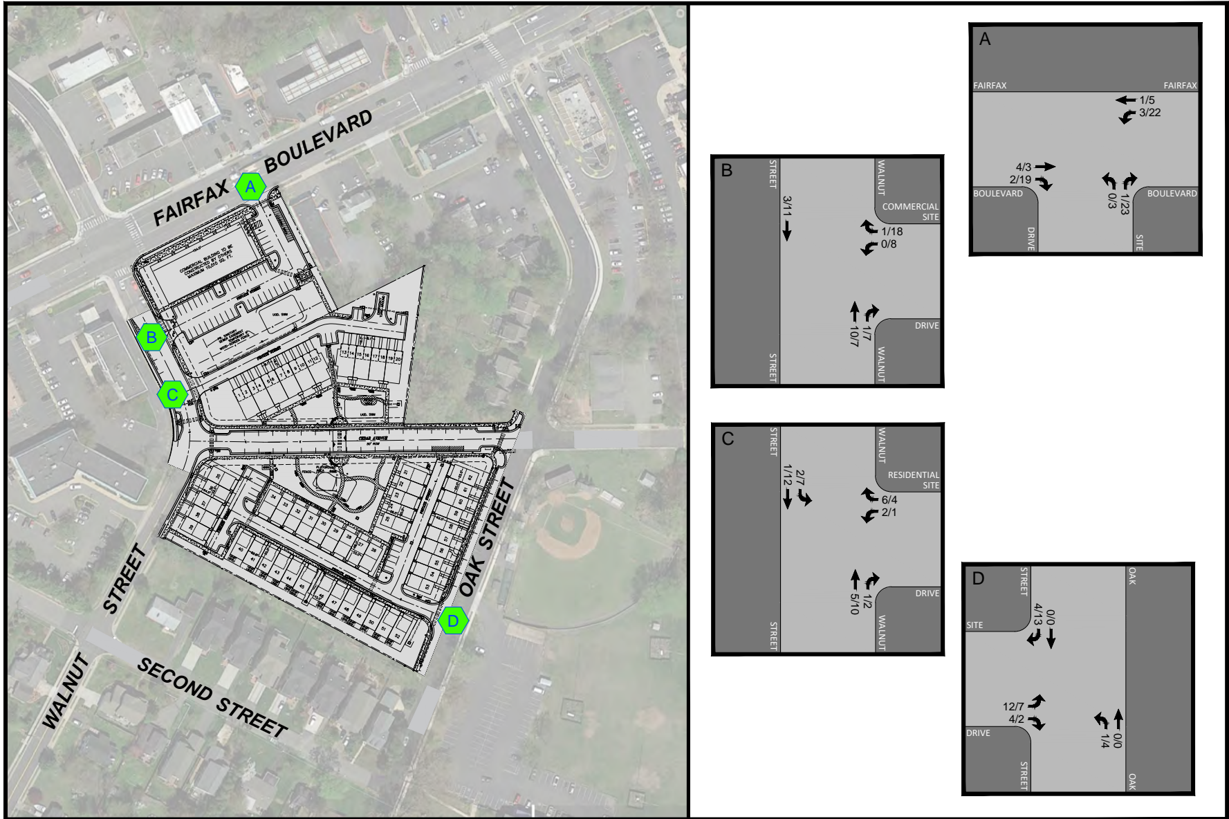
Figure 6-2B Site Traffic Assignments (Residential & Commercial) Site Driveways
