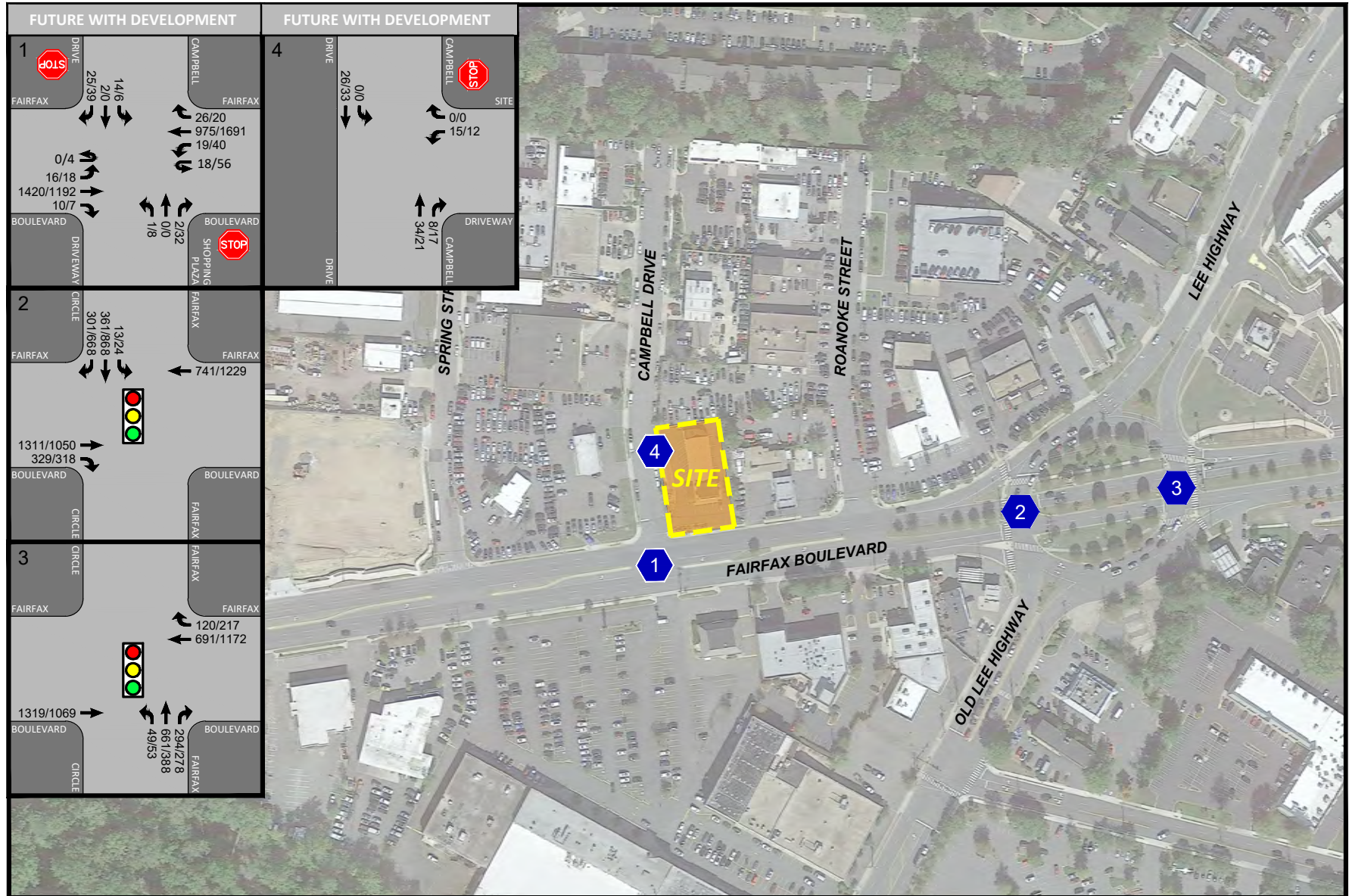
Figure 7-1 Future Conditions with Development Peak Hour Traffic Volumes
