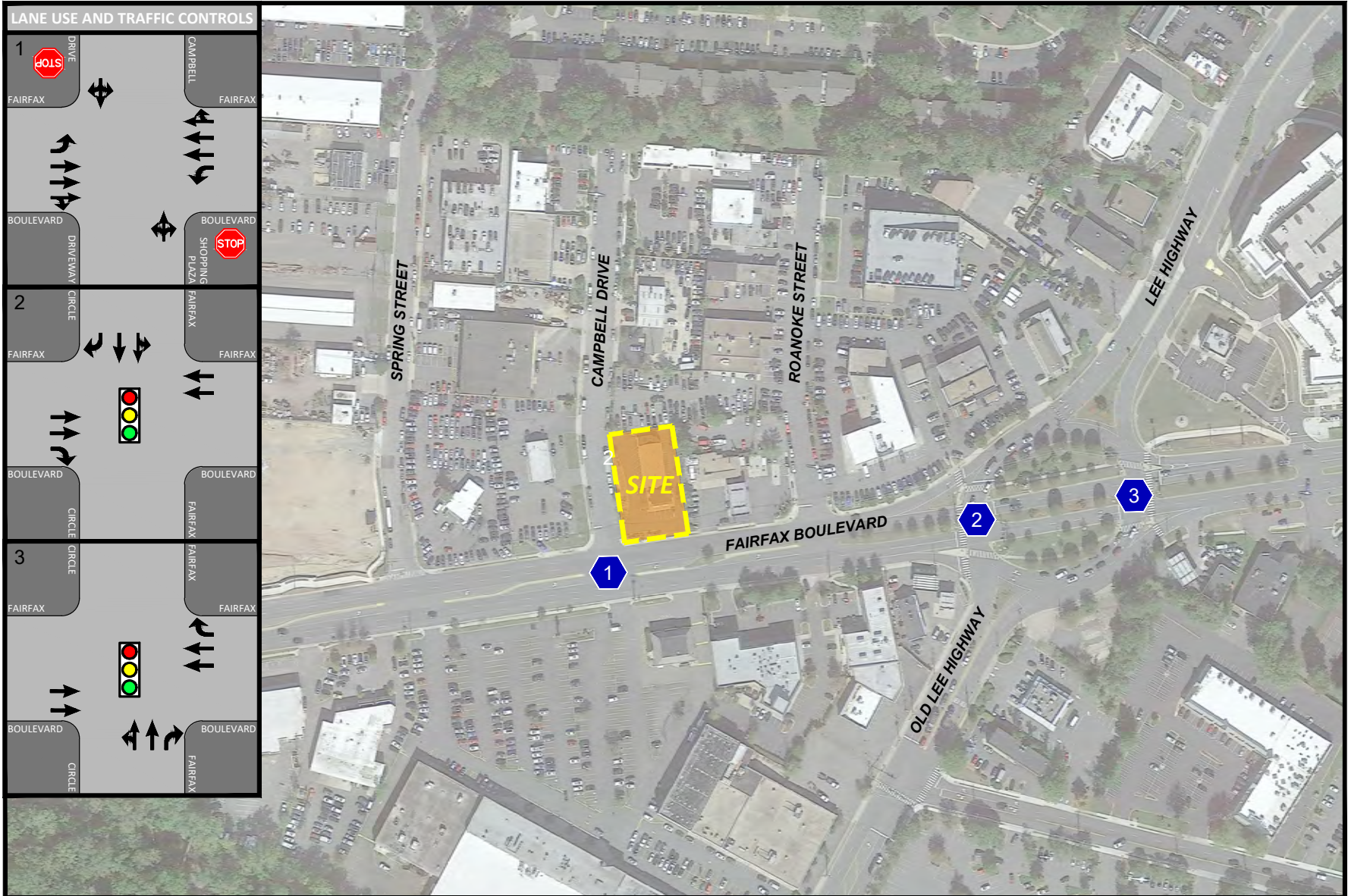
Figure 2-2 Existing Lane Use and Traffic Control
