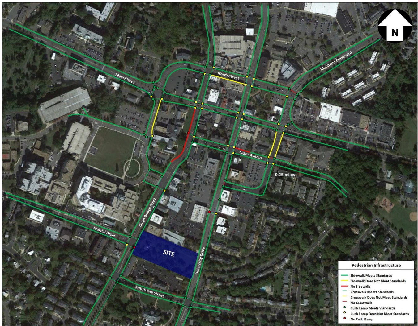
Figure 12: Existing Pedestrian Facilities
