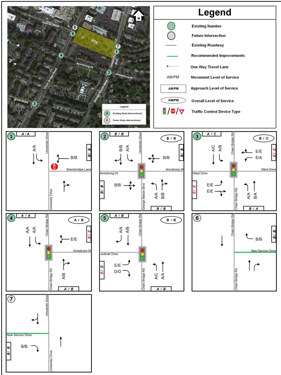
Figure 28: Future with Development (2026) – Levels of Service
