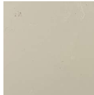
[WN5] ALUMINUM WINDOW SYSTEM FINISH: AKZONOBEL INTERPON POWDER COATINGS COLOR: CUSTOM COLOR TO MATCH BENJAMIN MOORE - BERBER WHITE (#995)
