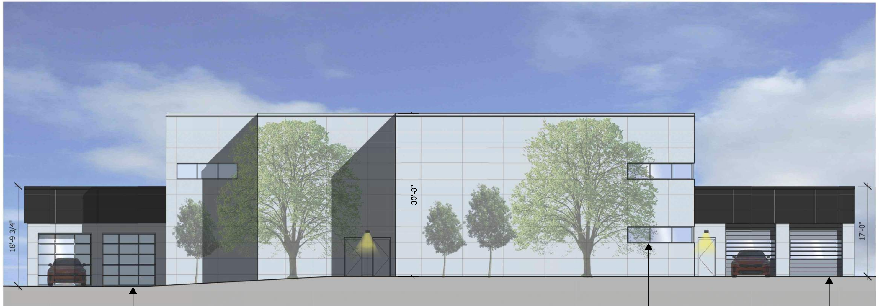
D-4 OVERHEAD DOOR - FULL VIEW COPLAY: MODEL 904 - FULL CLEAR GLASS W/ CLEAR ANODIZED ALUMINUM
