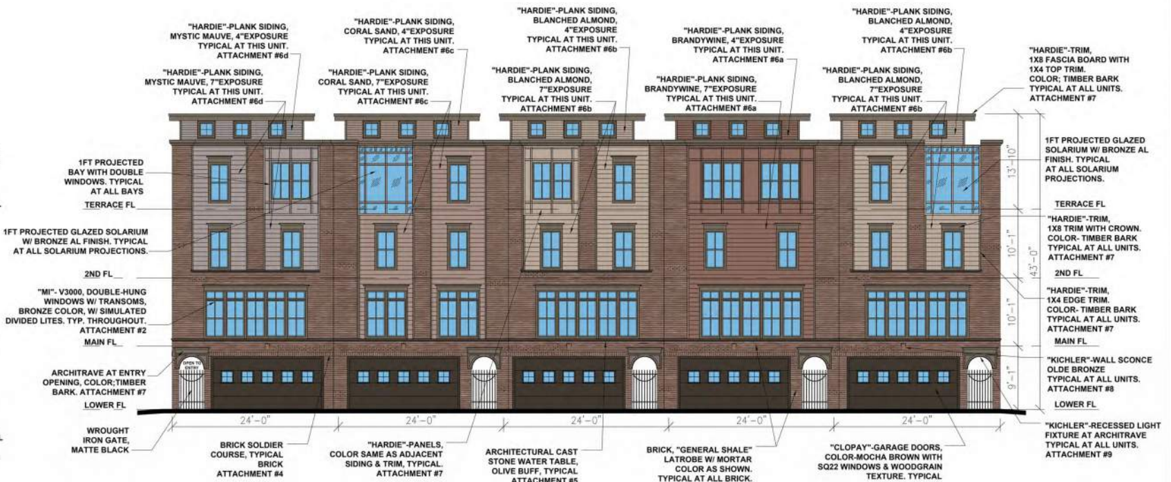
FRONT ELEVATION AT FIVE UNIT GROUPING
