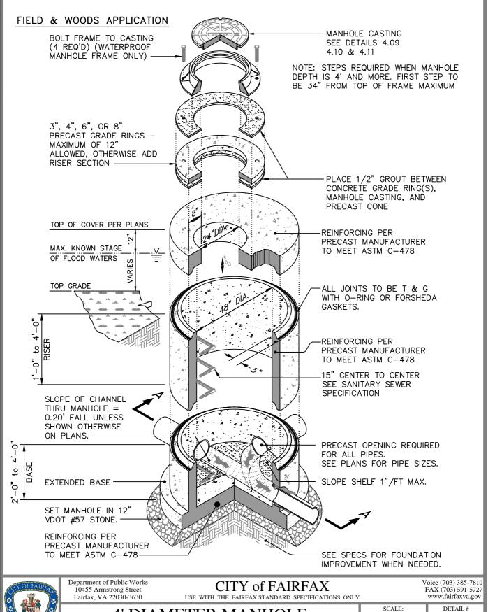
4' DIAMETER MANHOLE FLAT TOP | SCALE: | DETAIL # |
