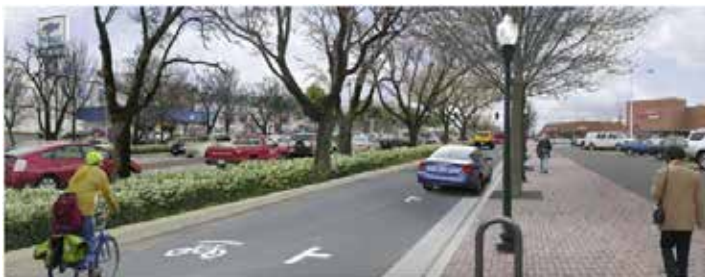
Implementation of the 5+2 lane configuration (5 through lanes with local lanes on either side), where appropriate, will make Fairfax Boulevard more pedestrian-friendly, while still accommodating vehicles.
